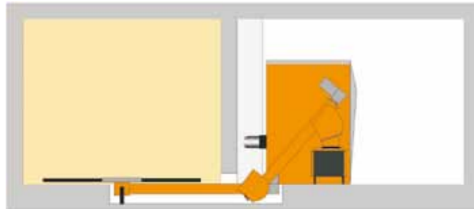
Silo clearing with inclined screw recessed in floor
