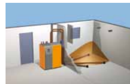
Pellet store room with suction pipes
